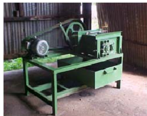
Prototype of the roller crasher
